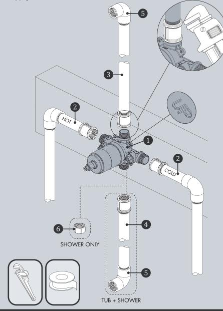
NOTE: The hot water supply lines go into the H inlet, and the cold water supply lines go into the C inlet. Do not use PEX or CPVC between the valve and spout.
