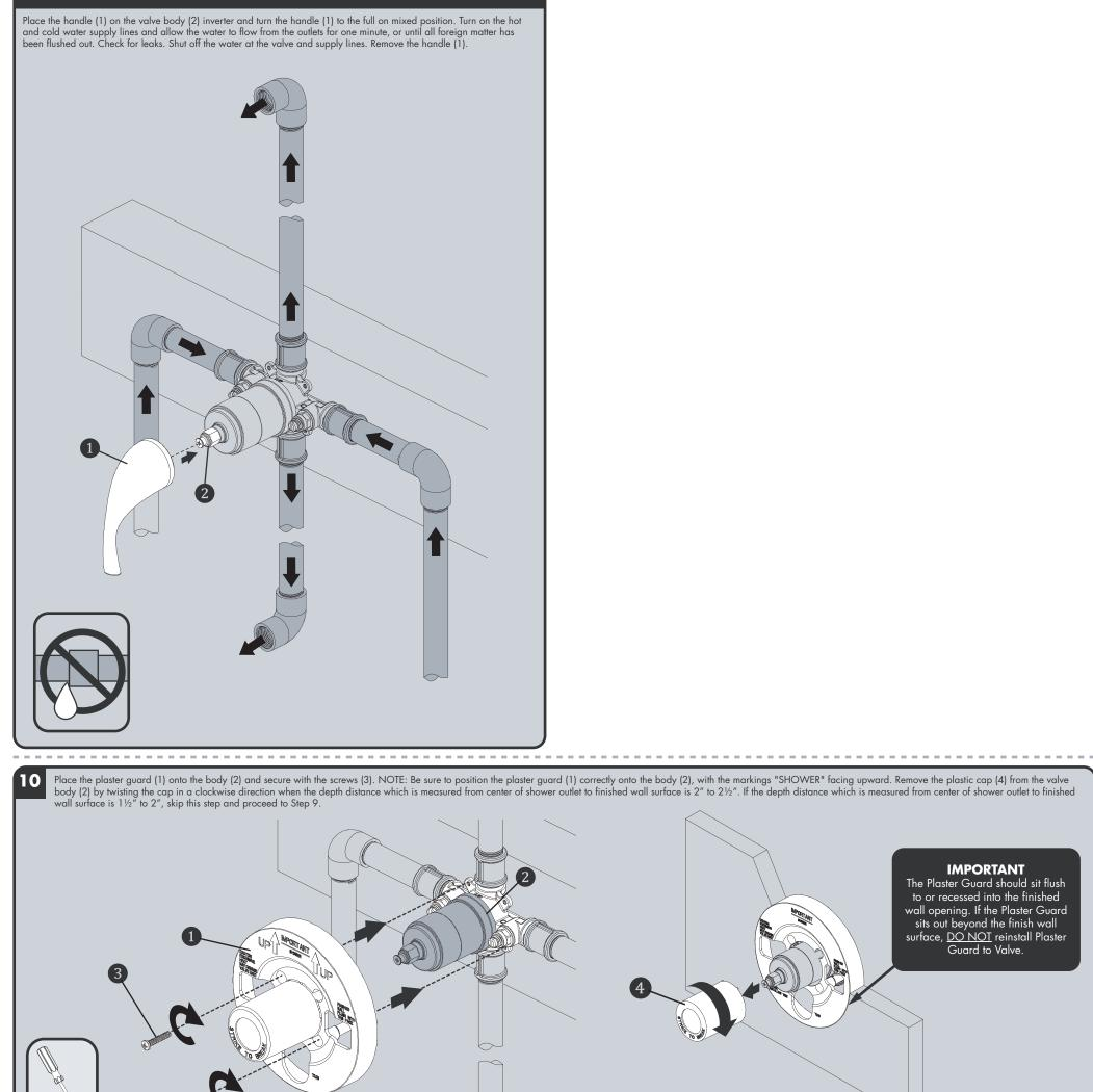
**IMPORTANT** The Plaster Guard should sit flush to or recessed into the finished wall opening. If the Plaster Guard sits out beyond the finish wall surface, <u>DO NOT</u> reinstall Plaster Guard to Valve.
