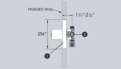
NOTE: Be sure to position the body (2) correctly in the wall, with the markings "UP" facing upward.
