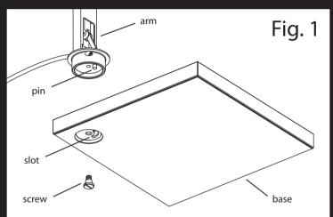
Insert the arm into the hole on the base, so that the pin fits into the slot. Use the screw to attach the arm to the base from the bottom. Tighten with a flat-head screwdriver. (Fig. 1)
