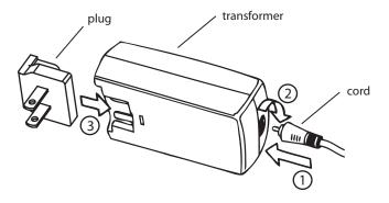
Insert the end of the cord into the transformer (1), and lock by rotating 90 degrees (2). Insert the plug to the transformer, being sure that it snaps firmly into place (3). (Fig. 2)
