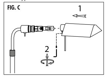
3. Plug in power cord. The High-Low Switch is located on the underside of the Socket Tube.
