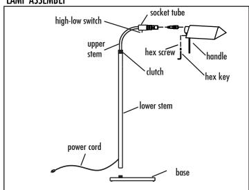
1. Push lower stem onto base and secure with set screw (Fig. A)
