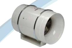
**Low profile** mixed flow fans, manufactured in plastic material (up to model 200) or in **galvanized steel** sheet protected with Epoxy paint (model 250 and 315), with external terminal box, removable motor-impeller assembly and adjustable single-phase motor, Class B, IP44.
