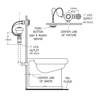
**NOTE:** Flush Connections shown in dotted line not included. **\*NOTE:** Valve can be installed in ceiling above fixture.
