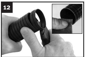
Cut the tube at the groove using a sharp utility knife to ensure a square, flat cut. Clean burrs from the cut end with emery paper.
