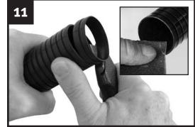
Cut the tube at the groove using a sharp utility knife to ensure a square, flat cut. Clean burrs from the cut end with emery paper.
