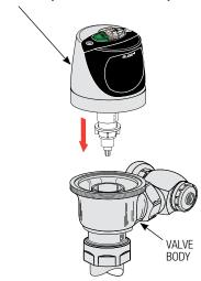
To facilitate installation, the 0-ring on the diaphragm assembly must be wet for easier insertion. NOTE: Sensor Lens must face directly forward. Rotating the Sensor to either side will decrease the Sensor's ability to detect a target.
