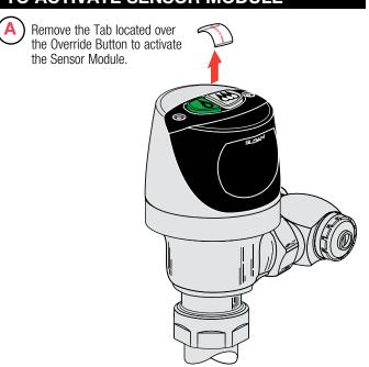
For the first ten (10) minutes of operation, a Visible Light flashes in the Sensing Window of the Sloan ECOS™ Electronic Dual Flush Flushometer when a user is detected.
