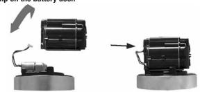
Disconnect wire clip from battery door and remove module from inner metal cover assembly.
