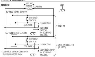
NOTE: A MAXIMUM OF TEN (10) SENSOR FLUSHOMETER UNITS CAN ACTIVATE FROM ONE (1) SLOAN EL-154 TRANSFORMER. CLASS 2 UL LISTED, 48 VA (MIN.) AT 24 VAC, PLATE MOUNTED.
