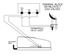
The remote receiver is to be connected to the millivolt valve. Connect one of the (2) 18 gauge wires from the 1410-A receiver to the TH terminal and the other to the THTP terminal on the terminal block on the millivolt gas valve.
