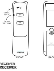
RECEIVER RECEIVER The transmitter operates on a 12V (A-23) battery (included). Install the 12V battery supplied with the unit into the battery compartment.
