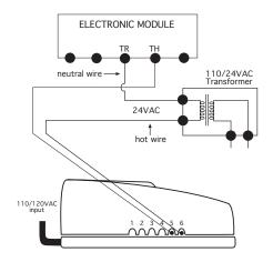
Most electronic systems operate on a 110 VAC/24VAC power transformer used to power the system electronic ignition module and electronic gas valve, which can be controlled by the 1410-A remote receiver as, illustrated.
