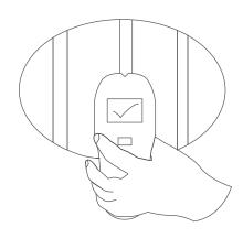
3. Determine the location for your mounting bracket, using the marked line for the top edge of the mirror and the marked stud locations as guidelines. Use a pencil to mark the location of the mounting holes. Ensure that the bracket is perfectly level before marking.
