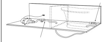
6. Secure the system's security device to the wall or a surrounding surface using the hardware provided.
