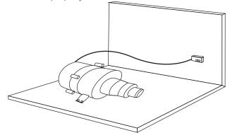
4. Connect one end of the 3' air hose to the blower motor outlet. Use a provided hose clamp to secure. Connect the opposite end of the hose to the security device, using another hose clamp to secure.
