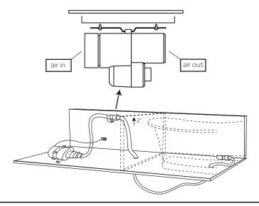
7. Plug the blower motor into its dedicated electrical receptacle. Proceed to Step 3 of installation to program your remote control.
