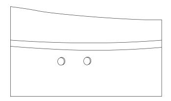
4. Mark the position of the magnets with a marker.
