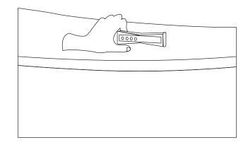
3. Position the magnets on the exterior of the bathtub, on the opposite side of the remote. The attraction of the magnets should catch onto the remotes magnets to determine their mounting location.
