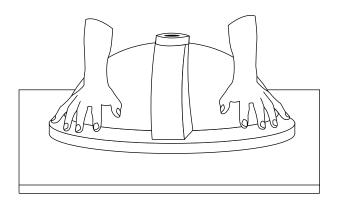
6. At each of the bolt holes in the counter top, attach sink clips by placing the long end of the bracket flat against the sink lip. Screw the wing bolts through the brackets and bolt holes and tighten.
