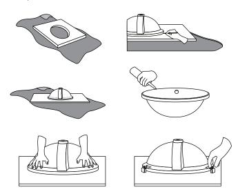
8. Carefully turn the counter top and sinks over. If needed, reposition the sinks by slightly loosening the wing bolts and adjusting.
