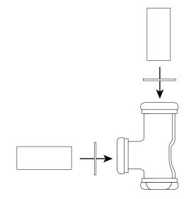
13. Attach the drain tube and flange to the waste and overflow tee with the sealing washer and slip nut. The beveled end of the sealing washer should face the tee.
