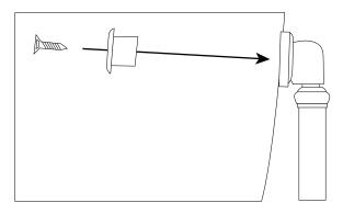
12. Attach the waste and overflow tee to the overflow assembly and shoe assembly with sealing washers and slip nuts. The beveled end of the sealing washer should face the tee.
