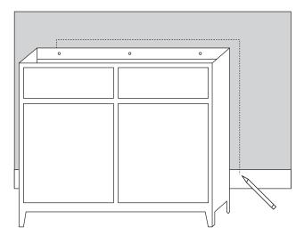
2. Locate and mark the location of the studs to which you will fasten your vanity. You can locate studs by using a stud finder.
