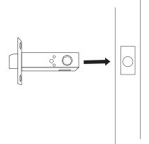
2. Use the latch bolt plate as a template to mark and drill pilot holes for the mounting hardware.
