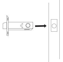
2. Use the latch bolt plate as a template to mark and drill pilot holes for the mounting hardware.
