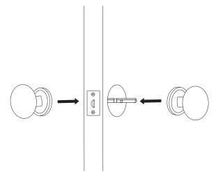
6. Hand thread the mounting hardware through the exterior door knob and tighten firmly with a screw-driver.
