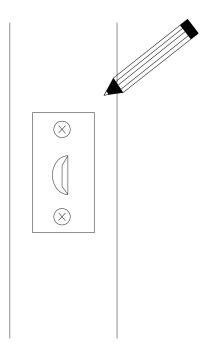
3. Insert the latch bolt and secure with two wood screws.
