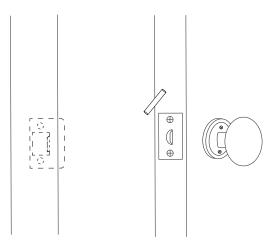
8. Position the strike plate on the door frame. The curved edge should touch the curved edge of the latch bolt when the door is closed. Then, secure the strike box and strike plate to the door frame with the remaining wood screws.
