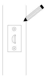
3. Insert the latch bolt and secure with two wood screws.
