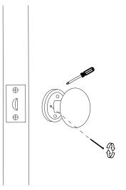
8. Place a small amount of paint or chalk on the end of the latch bolt. Then, close the door and turn the knob several times to transfer the paint onto the door frame to mark the strike plate location. Then, secure the strike box and strike plate to the door frame with the remaining wood screws.
