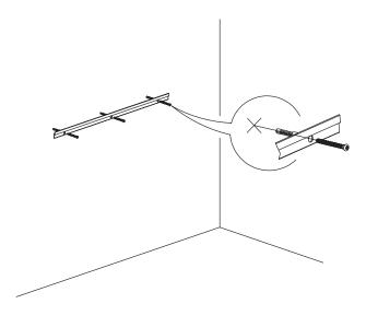
3. Attach the medicine cabinet to the mounting bar as shown, open the cabinet door, and make a mark on the wall with a pencil through the backplane hole (A).
