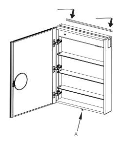
4. Remove the medicine cabinet, drill the mounting hole in the wall in the marked position, and place the wall anchors.
