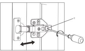
Rotate Clockwise: Distance between door and cabinet reduces. Rotate Counterclockwise: Distance between door and cabinet increases.
