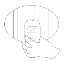
3. Determine the location for your mounting bracket, using the marked line for the top edge of the mirror and the marked stud locations as guidelines. Use a pencil to mark the location of the mounting holes. Ensure that the bracket is perfectly level before marking.
