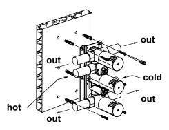
1. Install the valve body. Wrap the threaded portion of the joints in Teflon tape and connect the water inlet and outlet.
