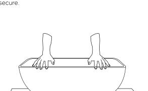
3. If desired, apply a continuous bead of silicone sealant around the perimeter of the sink base for additional stability.
