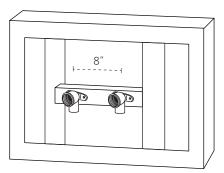
PROCEED WITH THE CONSTRUCTION OF THE FINISHED WALL. ONCE THE FINISHED WALL HAS BEEN COMPLETED, RESUME FAUCET INSTALLATION.
