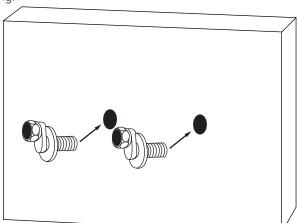
3. Insert one of the provided rubber O-rings into each of the faucet inlets, as shown. Connect the faucet to the installed wall couplers. Apply plumbers tape or thread sealant to the threads before attaching. Tighten firmly.
