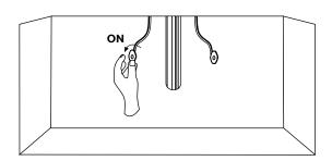
6. Remove the aerator from the spout and turn the faucet on. Ensure that both hot and cold water are running properly, and check for any leaks. Allow the water to flow for approximately 60 seconds to remove any dust or sediment within the water lines. Reattach the aerator.
