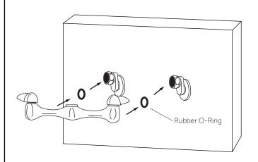
4. Attach the spout to the installed faucet body. Tighten the nut firmly using an adjustable wrench, but be careful not to overtighten.
