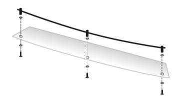
4. To mark the escutcheon placement, find the center point of the line that you drew on the wall. Make two marks to the right and left of the center, at an equal distance. The escutcheons should be 1-2" in from the outer edges of the glass shelf.
