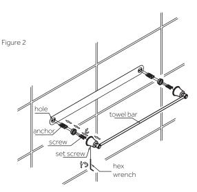
3. Insert anchors into the drilled holes. Fasten the mounting brackets to the wall, as shown, using the provided screws (Figure 2).
