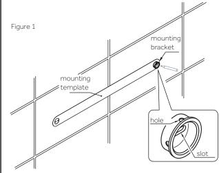
1. Position the mounting template on the wall at the desired installation location (Figure 1). Hold the mounting brackets in their location at each end of the template, and mark the location of the mounting holes. Make two marks in each slot, as each mounting bracket will require two screws. Ensure that the mounting template is level before making marks.
