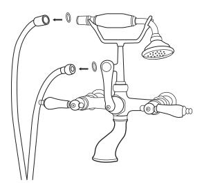
3. To complete the installation. connect the water supply lines (not included) to the faucet's inlets.
