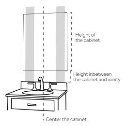
2. Locate and mark the position of the wall studs to which you will fasten your medicine cabinet. You can find studs by listening for a solid sound as you knock on the wall or by using a stud finder. If mounting holes are not pre-drilled, transfer these marks to the inside of the cabinet.
