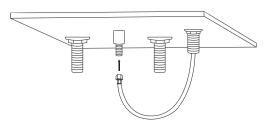
8. To attach the handles to the faucet, remove the decorative hot and cold indicators from each handle. Slide the handles onto each stem and tighten the screws to secure using a Phillip's screwdriver. Once secure, reinsert the hot and cold indicators.
