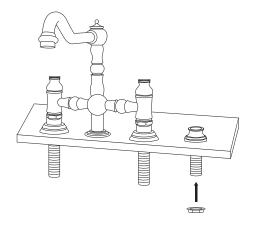
6. Insert the provided rubber O-ring into the end of the hand sprayer hose, and attach it to the hand sprayer assembly. Hand tighten firmly. Insert the hose and hand sprayer into its cradle from above the counter.
