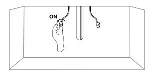
11. Remove the aerator from the spout and turn the faucet on. Ensure that both hot and cold water are running properly, and check for any leaks. Allow the water to flow for approximately 60 seconds to remove any dust or sediment within the water lines. Reattach the aerator and turn on the sprayer. Allow the sprayer to run for another 60 seconds, and check for any leaks.
