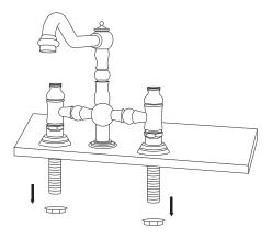
4. From below, secure the faucet to the counter by threading the provided lock nuts onto each threaded shank. Hand tighten, then finish tightening using a basin wrench.
