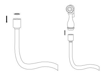
7. From beneath the counter, attach the hand sprayer hose by threading it onto the center post. Apply a bit of thread sealant or plumber's tape to the threads before tightening. Use an adjustable wrench to tighten firmly.
