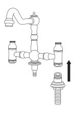
3. Remove the brass lock nuts from the threaded shanks and insert the faucet into its designated mount-ing holes on the mounting surface.
