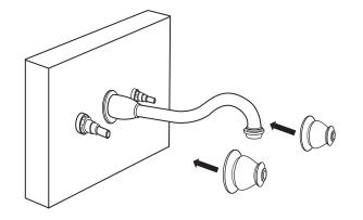
6. Attach the hot and cold handles to the valve stems, as shown. Ensure that the hot handle is on the left, and the cold is on the right.
