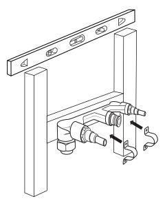
3. Attach the main water lines to the valve. Apply thread sealant or plumber's tape to the threaded connection to ensure a watertight seal.
