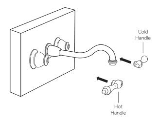
7. When your installation is complete, turn on the main water supply. Remove the aerator from the spout. Turn the water on to allow any dust or loose sediment to clear the system. Allow the water to flow through the spout for approximately 60 seconds, and verify that hot and cold water are running properly. Reattach the aerator once testing is complete.
