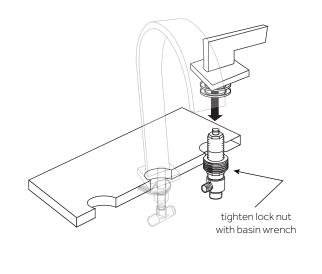
7. Repeat steps 5 & 6 to install the 'hot' valve stem into the left-side faucet hole.
