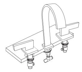
8. Use the provided braided water lines to connect each stem to the spout's T-connector, as shown. Apply thread sealant or plumber's tape to each threaded connection. Use an adjustable wrench to tighten, but be careful not to overtighten.
