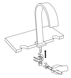
4. Thread the T-connector onto the end of the spout's threaded mounting post. Apply thread sealant or plumber's tape to the threads before tightening. Hand tighten firmly.
