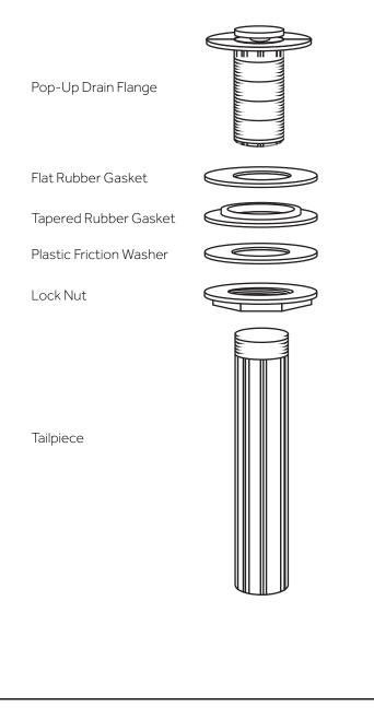
2. Apply plumber's tape to the threading on the tailpiece, then reattach the tail piece to the pop-up drain flange.
