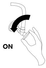
12. Once drain installation is complete, turn the faucet on for approximately 60 seconds to check for any leaks. Test both hot and cold water to ensure they are running properly.
