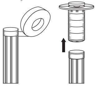
3. Slide the flat rubber gasket up the tailpiece until it meets the lip of the pop-up drain flange.
