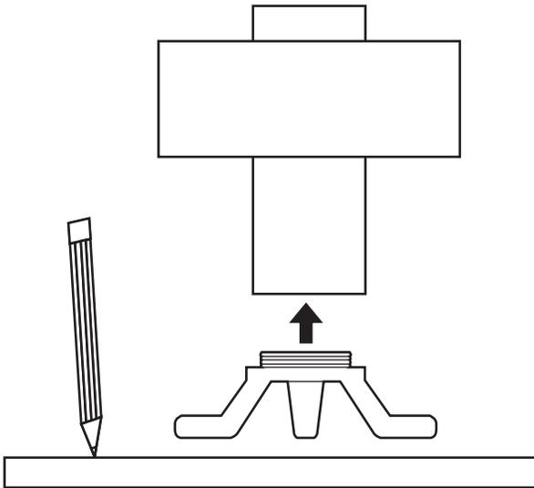
3. Drill pilot holes into the floor at the marked mounting hole locations.
