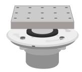
3. Place pea gravel over the drain flange coupling weep holes and around the perimeter to prevent mortar from filling and blocking the holes.
