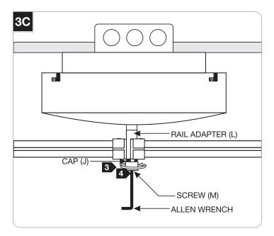
**3** Replace and tighten the cap (J) to the rail adapter (L).
