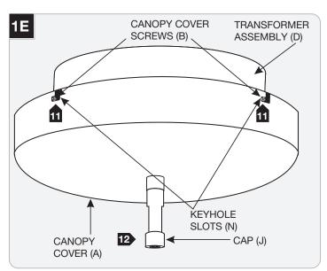
Replace the canopy cover (A) onto the transformer assembly (D). Line the keyhole slots (N) with the installed canopy cover screws (B). Rotate canopy cover (A) counterclockwise so canopy cover screws (B) are located at the bottom left hand section of the keyhole slot (N). Tighten the two canopy cover screws (B). Install third canopy cover screw (B) through oval shaped hole to secure canopy cover (A).
