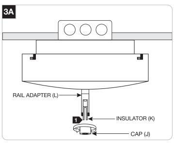
Remove cap (J) from rail adapter (L). Remove the insulator (K).
