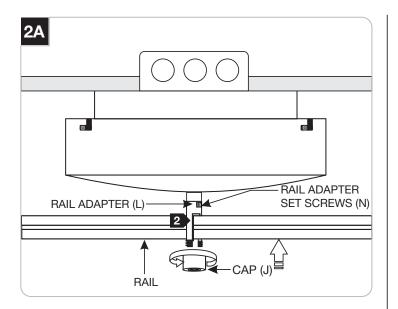
1 Before installing the rail you will need to adjust the height of your rail support adapter so it matches the transformer rail adapter (L). To adjust the height of the transformer's rail adapter, loosen the rail adapter set screws (N) with the supplied allen wrench. You may slide the rail adapter (L) down the stem, and resecure it by tightening the set screw (N). The transformer's rail adapter can only be adjusted to increase the height of the rail adapter.
