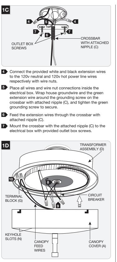
Note: The #95305 surfacemount transformer has 3 holes in the transformer assembly (D). If applicable you may install 3 screws (not supplied) to provide additional support.
