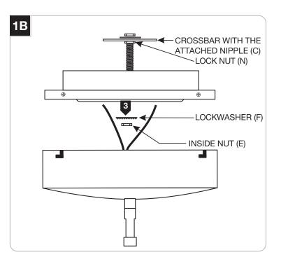
3 Remove the inside nut (E) and lockwasher (F) to remove the crossbar with the attached nipple (C). DO NOT REMOVE the nipple from the crossbar. The nipple may be adjusted if the installed junction box is not at a normal height. Loosen lock nut (N) to adjust nipple.
