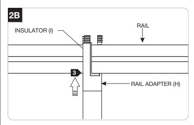
From bottom of the rail push the rail adapter (H) all the way onto the rail so that the rail fits in the insulator (I).
