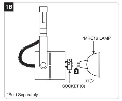
While holding the socket (C) with one hand, carefully insert the MRC16 lamp into the socket (C).
