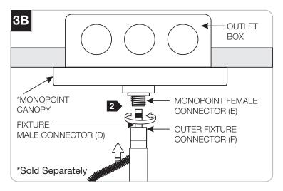
Insert fixture male connector (D) into monopoint female connector (E). Thread the outer fixture connector (F) to the monopoint female connector (E) to secure.
