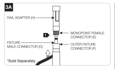
1 Unthread rail adapter (H) from male connector (D)
