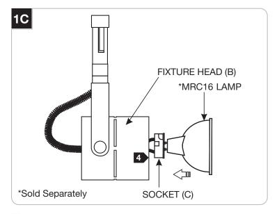
Place the Socket (C) and MRC16 lamp into the fixture head (B).
