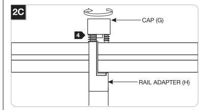
Replace and tighten the cap (G) to the rail adapter (H).
