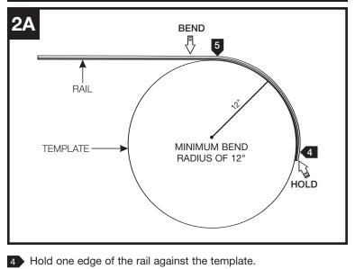
5 Start bending the rest of the rail along the template until the desired curve is achieved.
