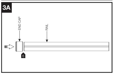
6 Gently tap the end cap completely onto each open end of the rail.
