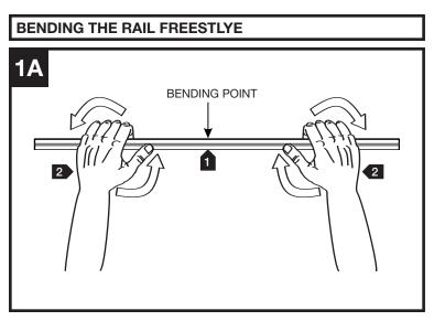
Choose the center of bending section on the rail. The bending point should be centered between the hands.
