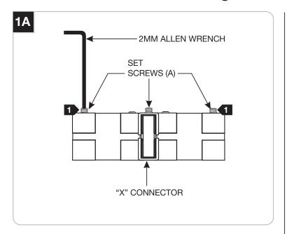
Clear the connector ends by backing out (DO NOT REMOVE) the four set screws (A) with the provided 2MM Allen wrench.
