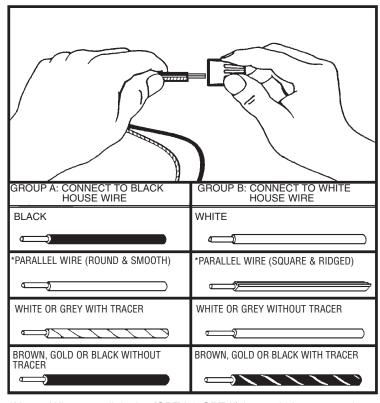
\*Note: When parallel wire (SPT I & SPT II) is used, the tracer wire is square shaped or ridged and less tracer wire is round in shape or smooth. (Seen best when viewed from wire end.)
