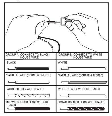
\*Note: When parallel wire is used, the tracer wire is square shaped or ridged and less tracer wire is round in shape or smooth.
