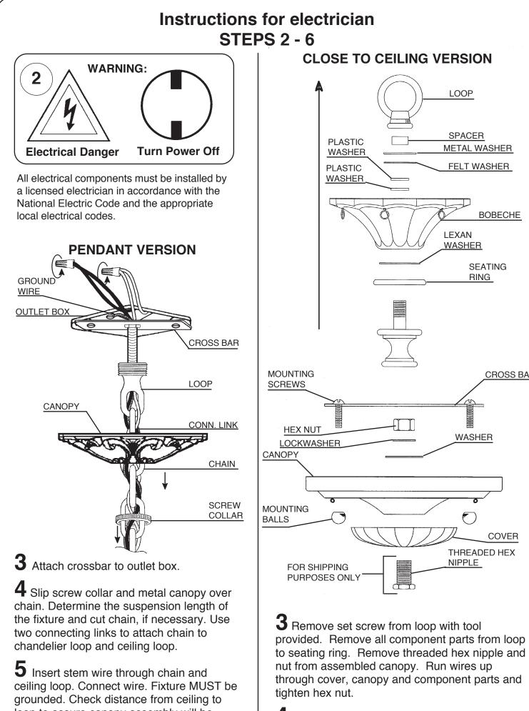
**4** Attach cross bar to outlet box. Connect wire.
