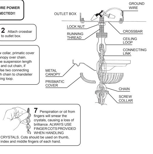
4 Insert stem wire through chain and ceiling loop. Connect wires. Fixture MUST be grounded.
