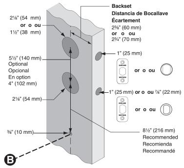
If necessary, cut out Throughbolt Template, mark door, and drill hole.
