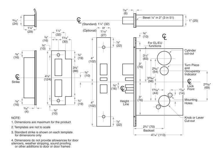
ANSI Standards: L9000-Series locks meet all requirements for installations in doors and frames prepared in accordance with ANSI specifications A156.13, 2005
