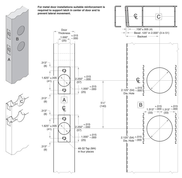
Dimensions shown in parentheses () are in millimeters
