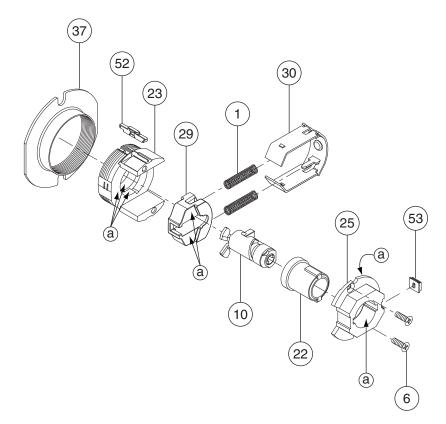
(a) Apply light film of 100% synthetic grease on surfaces with brush.
