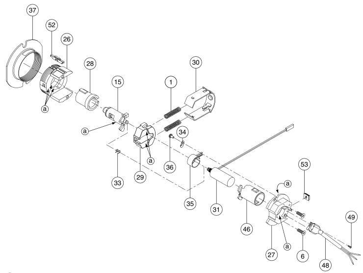
(a) Apply light film of 100% synthetic grease on surfaces with brush.
