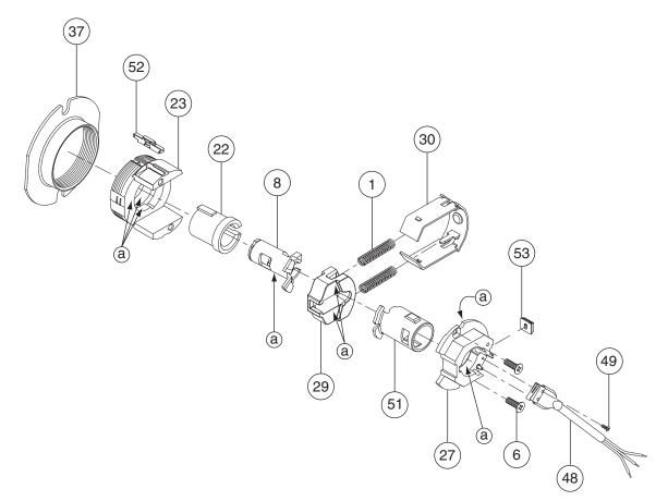
(a) Apply light film of 100% synthetic grease on surfaces with brush.
