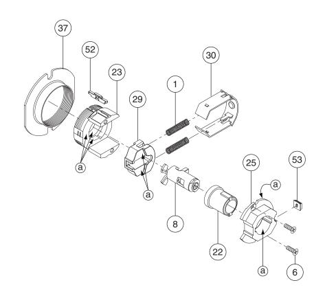
(a) Apply light film of 100% synthetic grease on surfaces with brush.
