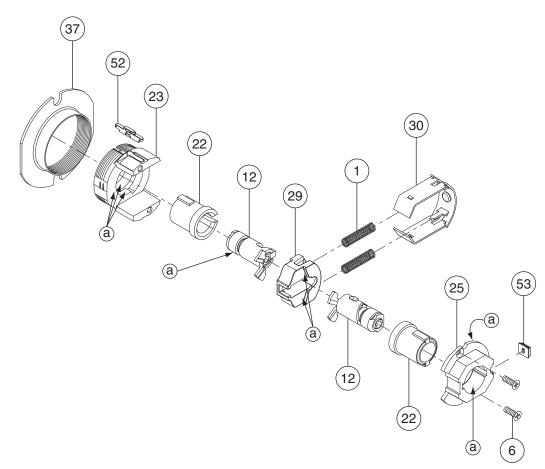
(a) Apply light film of 100% synthetic grease on surfaces with brush.
