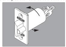
3b Insert latch into hole. Line up and trace around faceplate.
