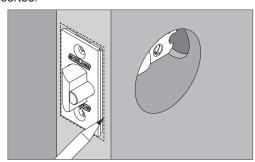
3c Install latch with provided screws.
