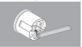
5b With key removed, insert cylinder into rings (See Step 1) and guide driver bar into slot in latch.
