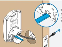
The bump on the tailpiece aligns with the slot in the bolt.
