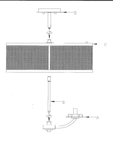
1. Carefully unpack and identify all parts referring to the illustration for parts identification.
