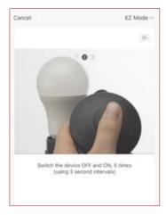
This device has advanced pairing retention technology. The device(s) that already paired will remain paired to the network, the device(s) that did not pair will return to pairing mode. To reset to factory settings, turn the switch off/on 8x.
