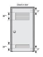
\* Required spacing. (External exhaust elbow requires additional space)
