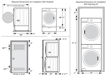
\*\* External exhaust elbow requires additional space. \* Required spacing
