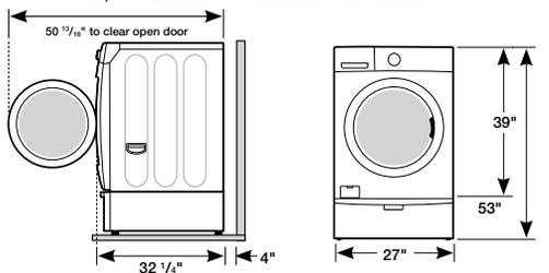
Required Dimensions for Installation With Stacking Kit
