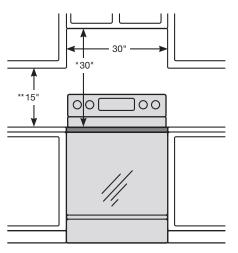
IMPORTANT: To eliminate the risk of burns or fire caused by reaching over heated surface units, cabinet storage space located above the surface units should be avoided. If cabinet storage is to be provided, the risk can be reduced by installing a range hood that projects horizontally a minimum of 5" beyond the bottom of the cabinets.
